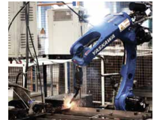
Robotic arm welding shelf joints
