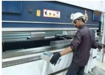
CNC controlled, automatic sheet bending machine
