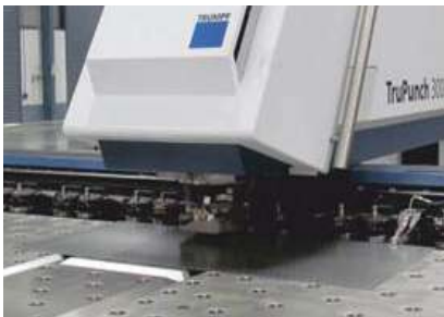
Automatic, CNC controlled sheet punching machine
