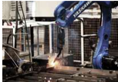
Robotic arm welding shelf joints
