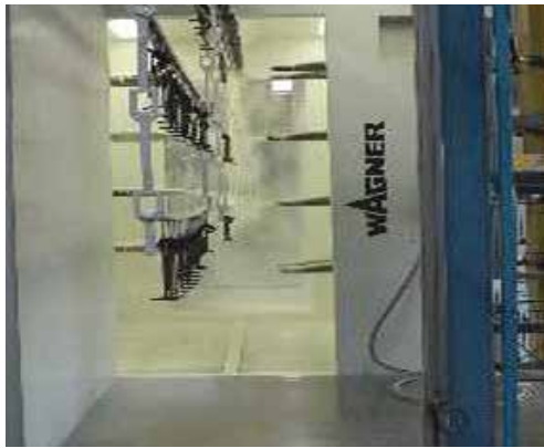
Fully conveyerised automatic powder coating plant
