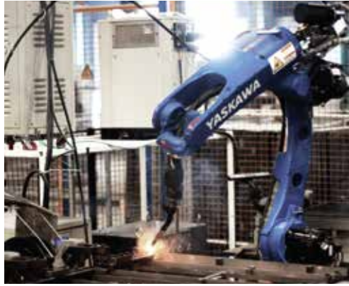
Robotic arm welding shelf joints
