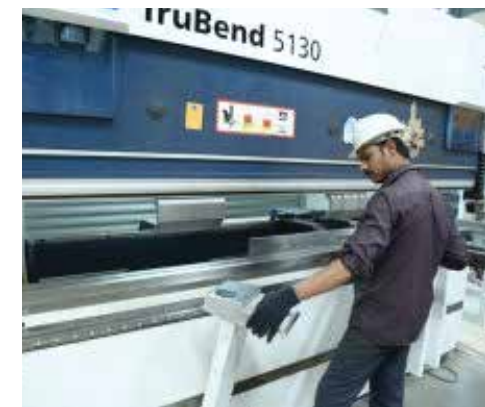
CNC controlled, automatic sheet bending machine
