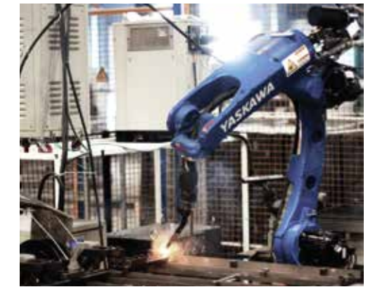
Robotic arm welding shelf joints
