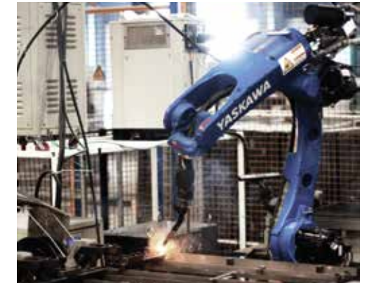
Robotic arm welding shelf joints
