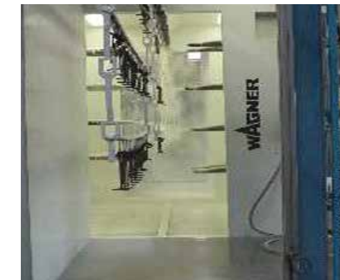
Fully conveyerised automatic powder coating plant
