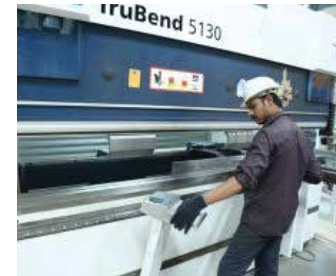
CNC controlled, automatic sheet bending machine
