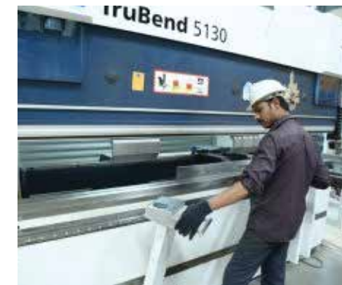
CNC controlled, automatic sheet bending machine
