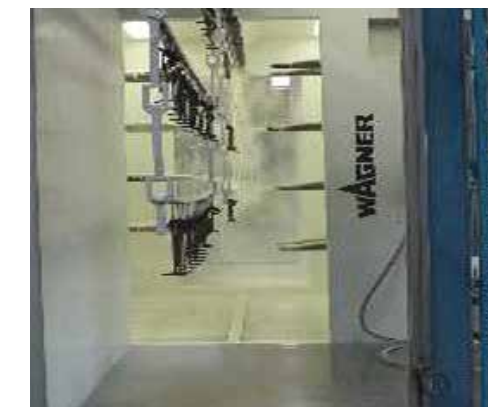
Fully conveyerised automatic powder coating plant
