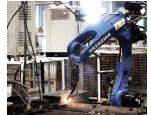
Robotic arm welding shelf joints
