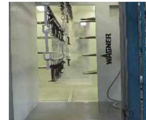
Fully conveyerised automatic powder coating plant
