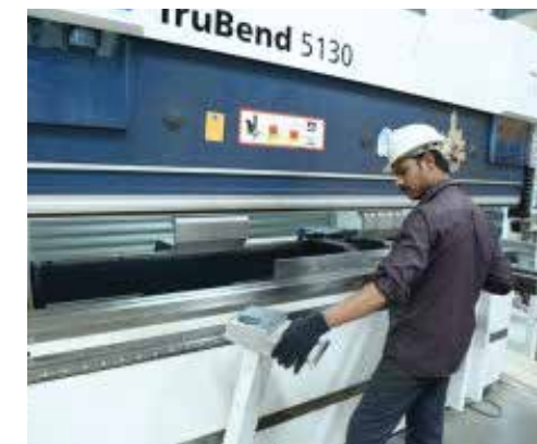
CNC controlled, automatic sheet bending machine
