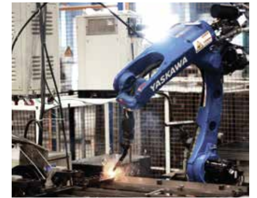
Robotic arm welding shelf joints
